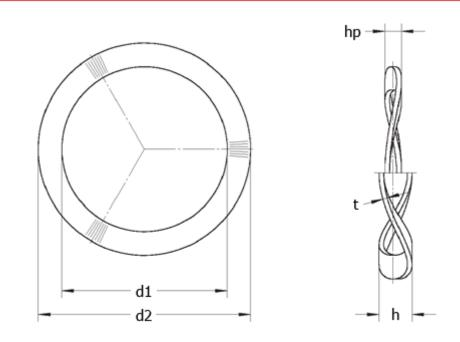
$\begin{array}{ll} d1 & = 102.00 \\ d2 & = 112.00 \\ F (N) at hp & = 520.0 \\ For bearing & = 6015, 16015 \\ h & = 4.7 \\ hp & = 2.05 \\ t & = 0.60 \\ Waves & = 7 \end{array}$
